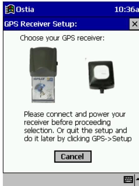
This screen will allow you to choose which GPS receiver you will be using and have the Ostia software automatically configure itself to work with that GPS receiver.
